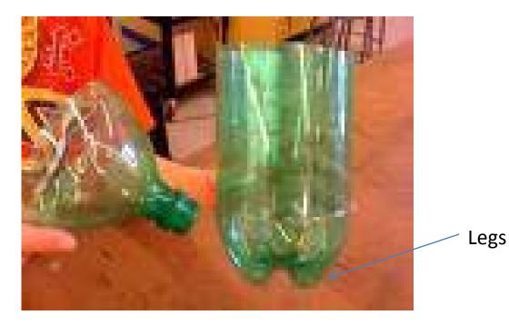
Cut the top off with a knife. Drill a quarter inch hole in the center of bottom . Then drill about eight 3/16 holes between and on the legs of the composter bottles. They should be about an inch above the bottom.
